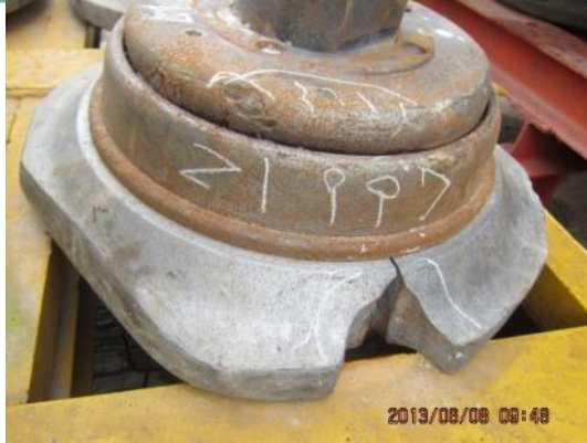
Impact damage to discs
