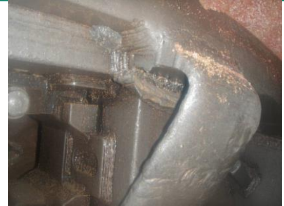
Damage to mixing and rock crusher arms, cutterhead
